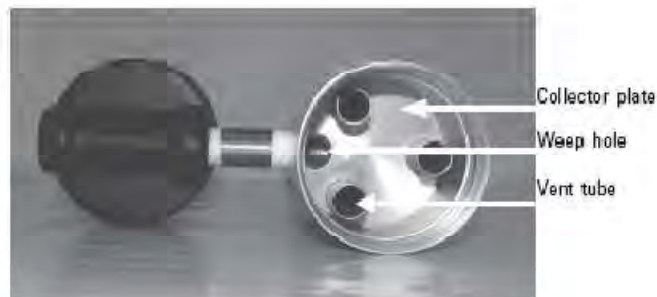
Figure 5-25. Inside of inlet collector assembly.
