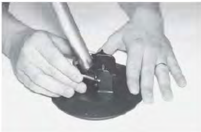
Figure 2-8. Placing the metal bracket on the tripod foot.
