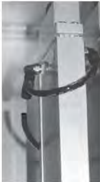
Figure 5-39. Main dryer vacuum line removed from T-fitting.
