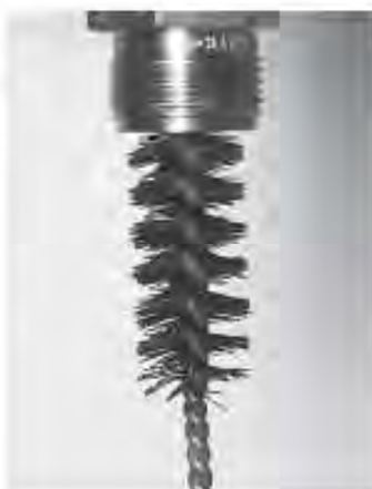
Figure 5-46. Cleaning the valve with the valve brush.
