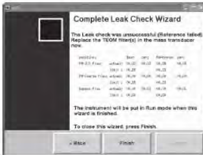
Figure 3-11. Leak Check Wizard finish screen with fail message.
