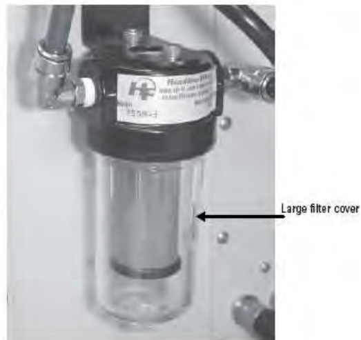
Figure 5-33. Bypass in-line filter.
