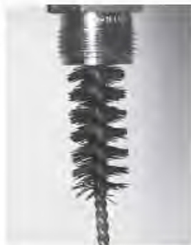
Figure 5-47. Cleaning the valve with the valve brush.
