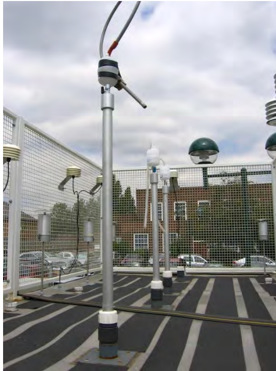
Figure 17: BX-302 zero filter during application in the field
