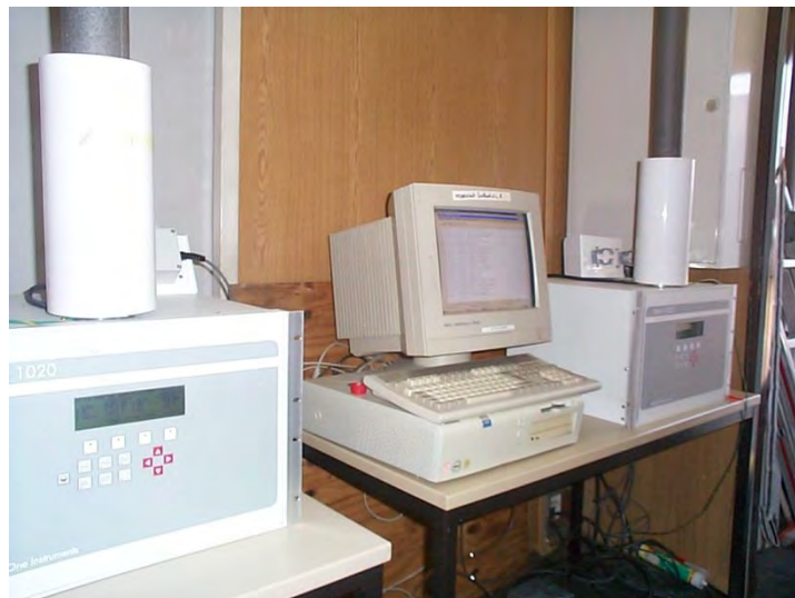
Figure 6: BAM-1020 measuring system, installed in measurement cabinet
