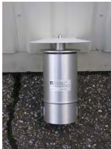
Figure 4: European PM10-sampling inlet BX-809 for BAM-1020
