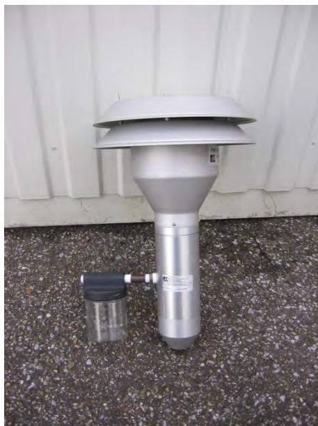
Figure 3: US-EPA PM 10 sampling head BX-802 for BAM-1020
