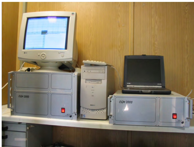
Figure 7: Test gas application by permeation system and computer for controlling
