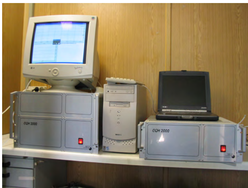
Figure 8: Test gas application by permeation system and computer for controlling
