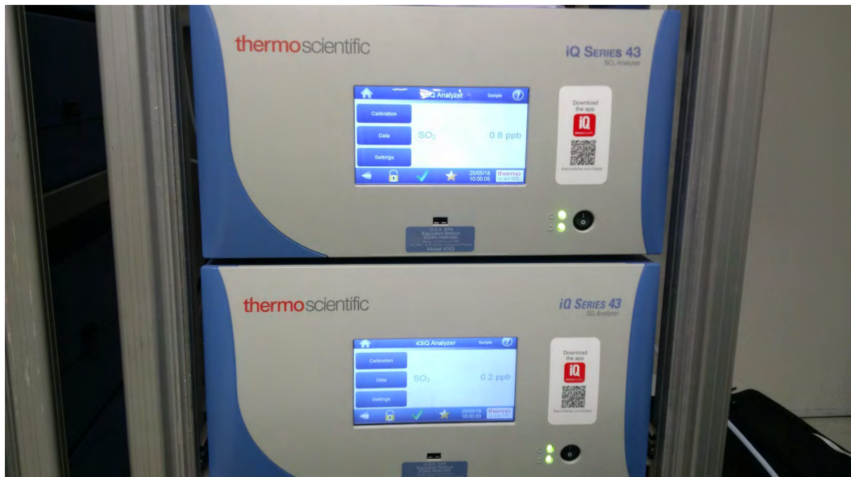
Figure 6: 43iQ test instruments with measured value display
