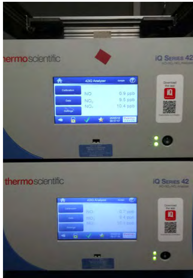
Figure 1: View of the 42iQ analyser
