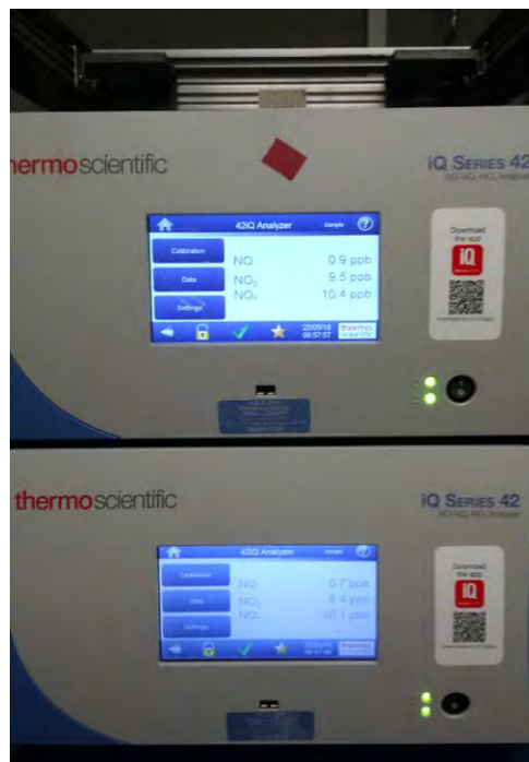
Figure 6: 42iQ test instruments c/w measured value display
