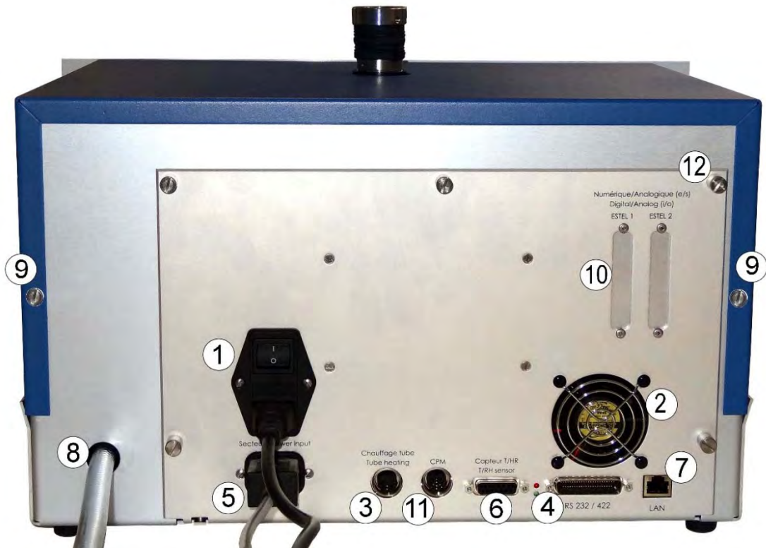
(1) general fuse F1 and mains power supply block, (2) fan, (3) TUCHEL connector for tube heating, (4) RS232/RS422 socket, (5) external pump supply, (6) external temperature and humidity sensors, (7) TCP/IP socket, (8) pump outlet, (9) holding cover screws, (10) ESTEL board options, (11) connection socket to CPM option, (12) holding screws of the rear panel drawer.
