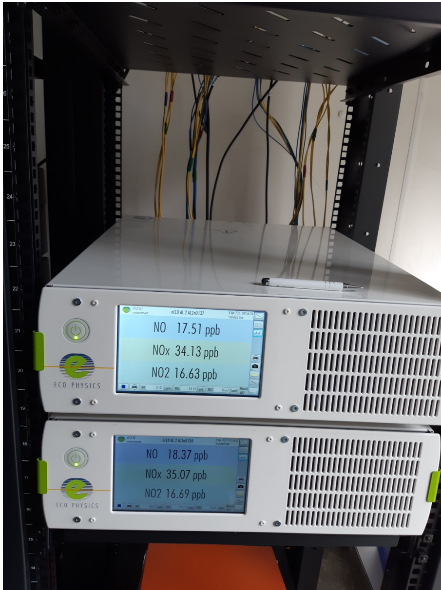
Figure 9: nCLD AL 2 in the measuring station during the field test
