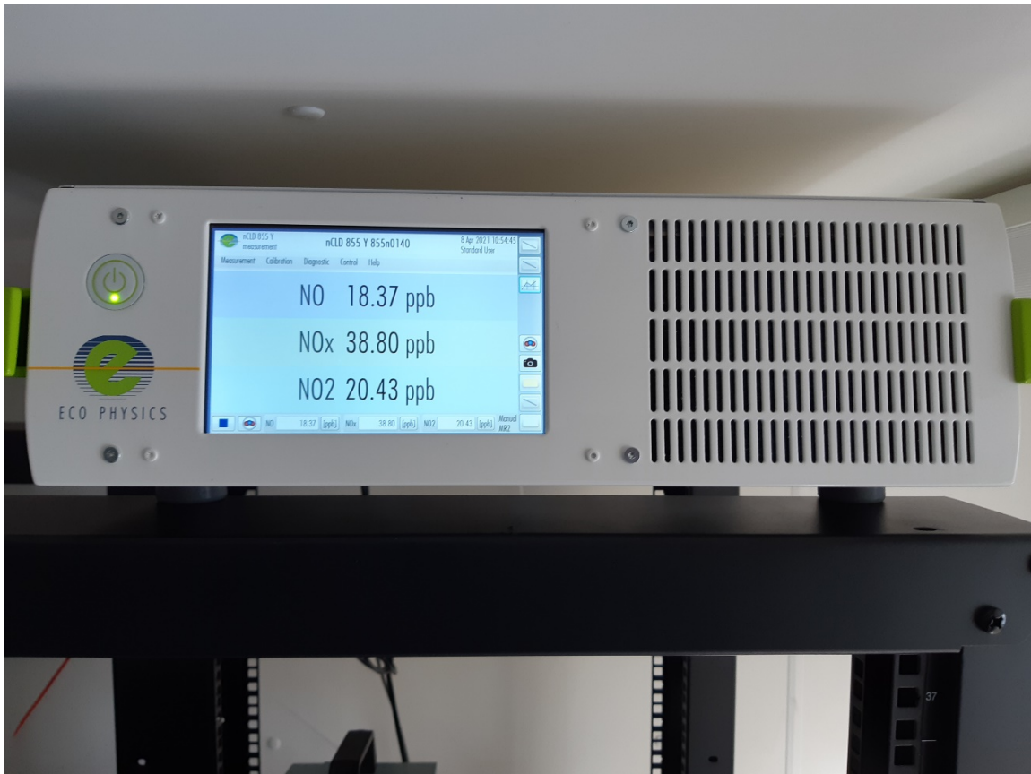
Figure 6: nCLD 855 Y in the field measuring station
