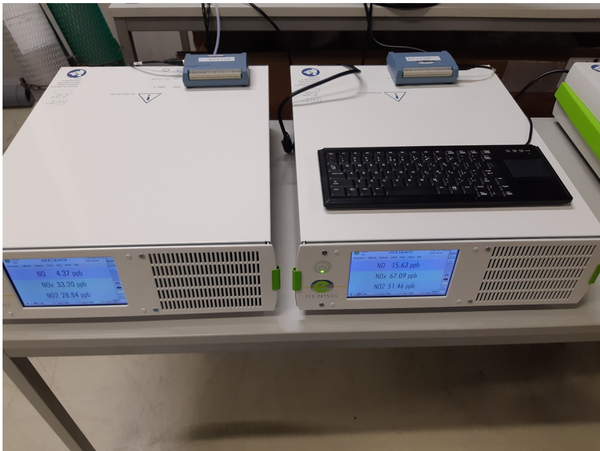
Figure 1: View of the nCLD AL 2 analyser
